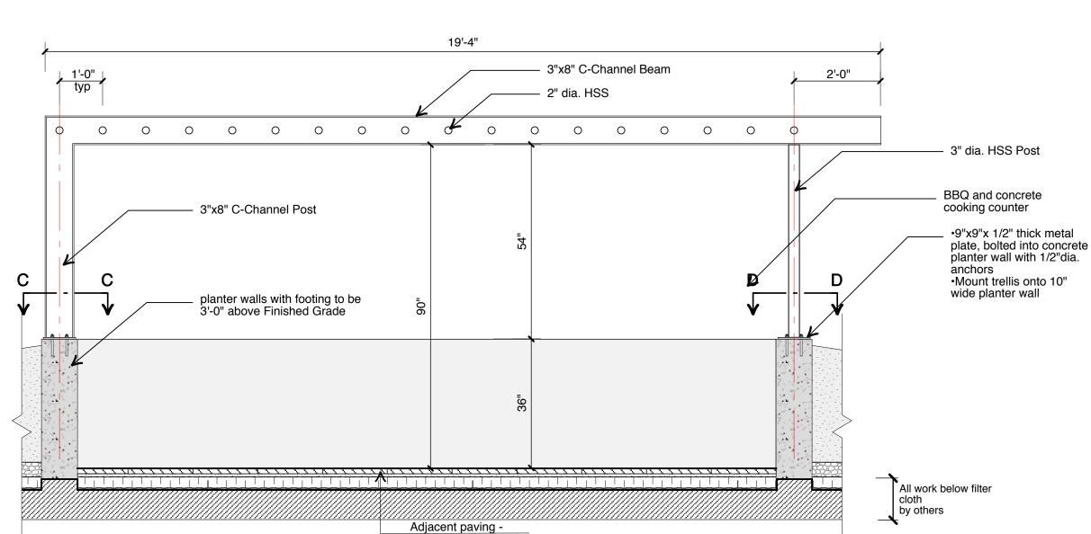
9" sq. 1/2" thick steel plate bolted onto 10" wide cip. concrete wall secured into concrete slab
