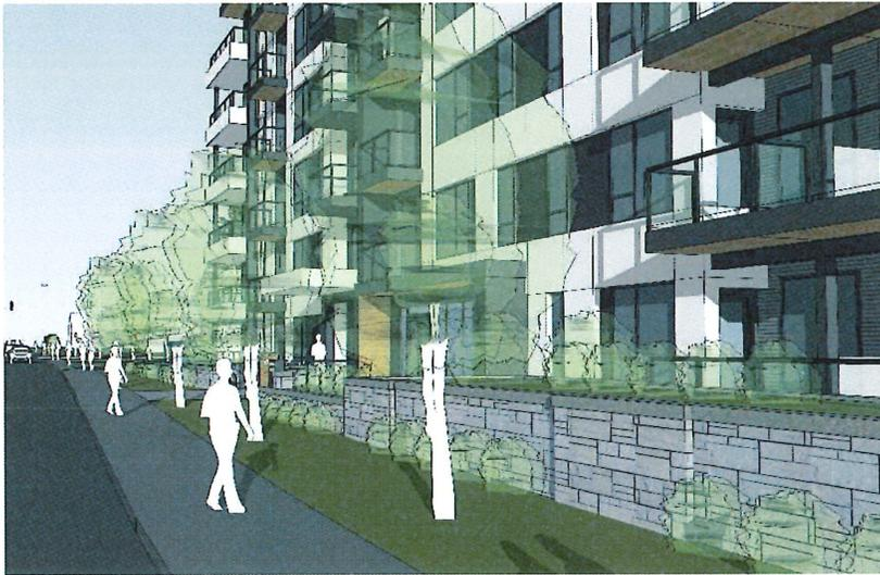
Along the South of the site, the lane had been roughly modeled which contributed to the perception of tall planter walls. With accurate lane grades and deeper soil for rainwater, the planter wall is on average 1m tall. The planter being continuous allows for better screening and separation from the lane, versus interrupting the planters with adding a walkway and steps.
