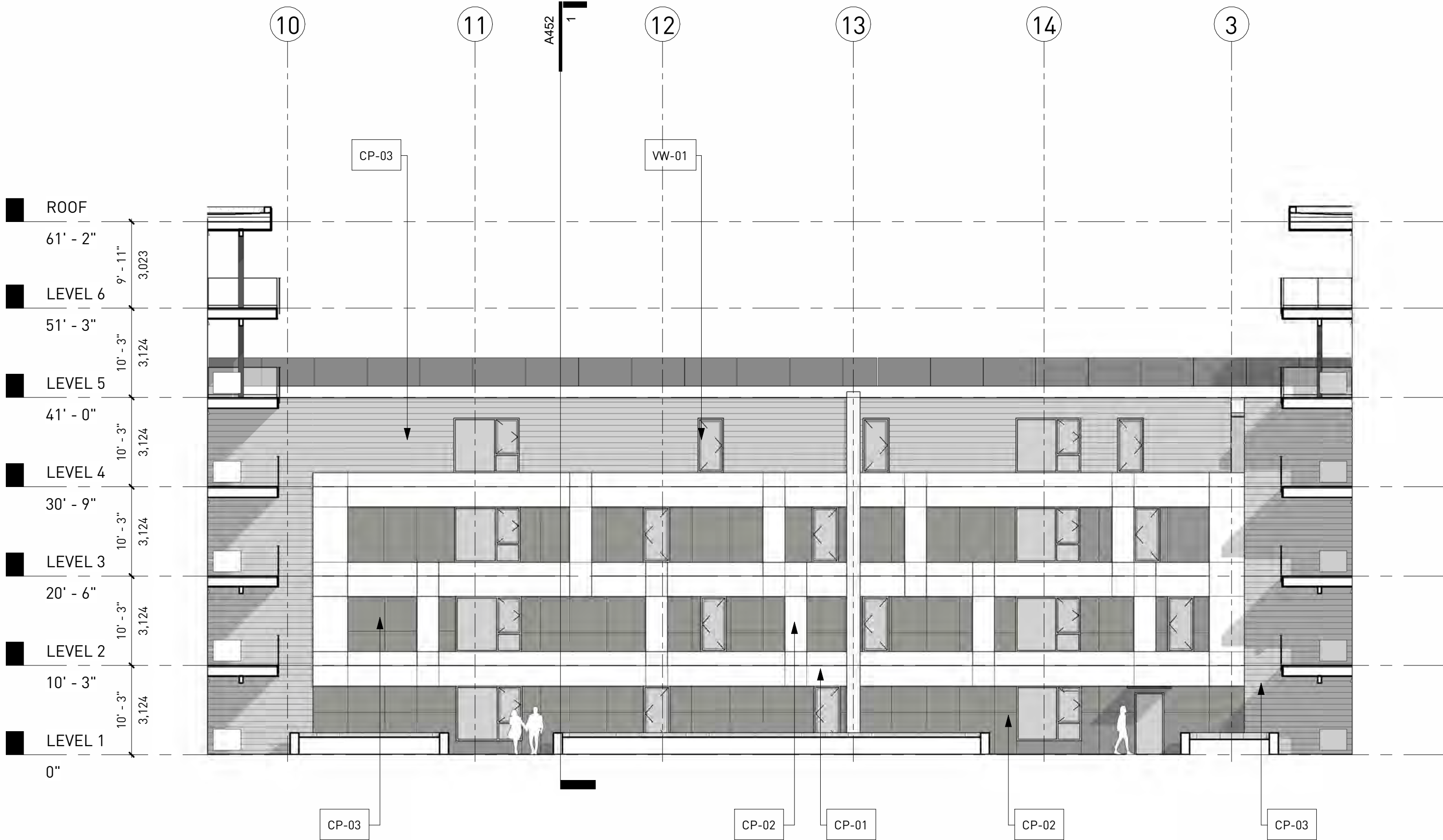
3 South Courtyard Elevation 3/32" = 1'-0"
