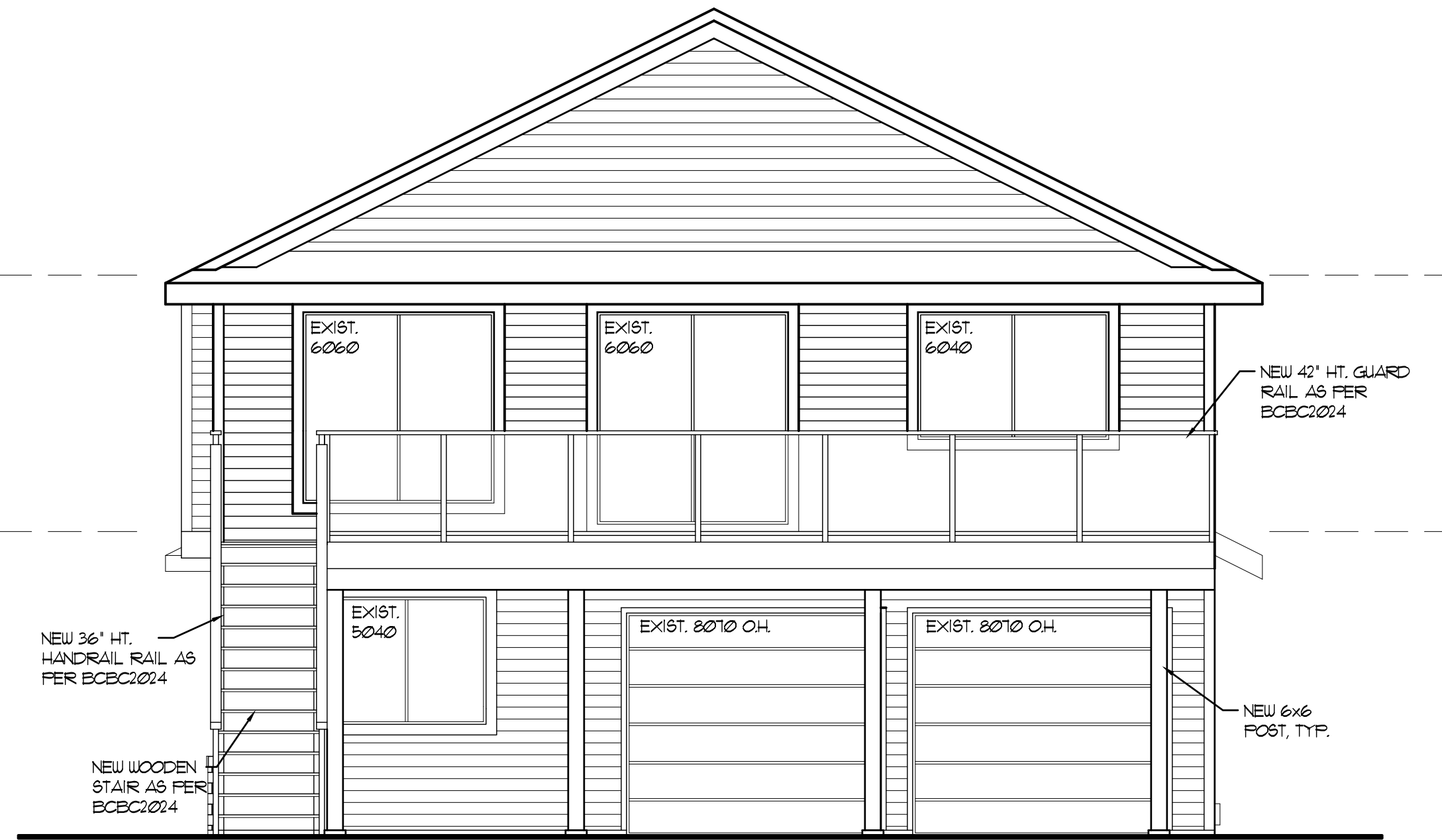
NEW REAR ELEVATION SCALE: 1/4" = 1'-0"
