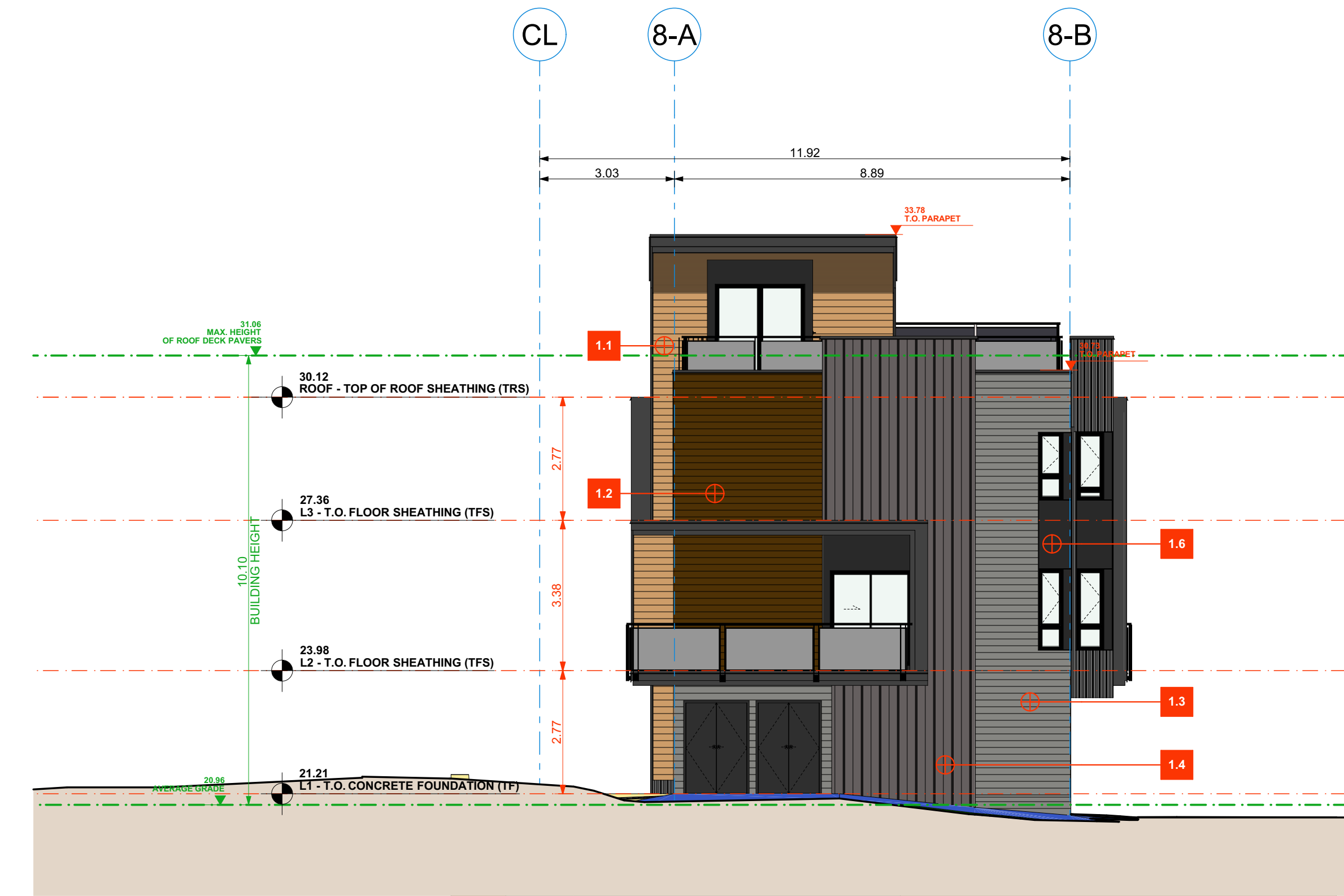
2 Building 2 - West Elevation SCALE: 1/8" = 1'-0"
