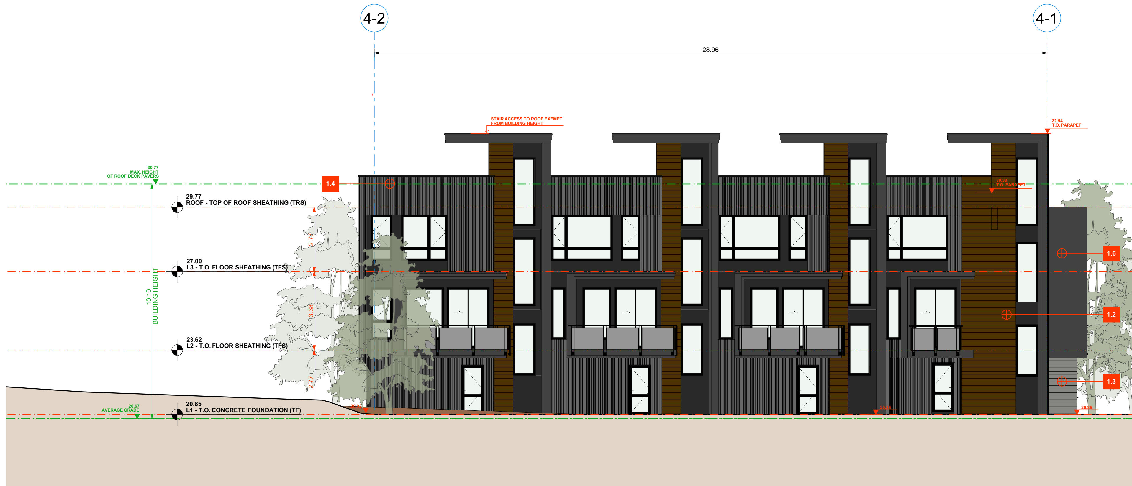
3 Building 5 - North Elevation SCALE: 1/8" = 1'-0"
