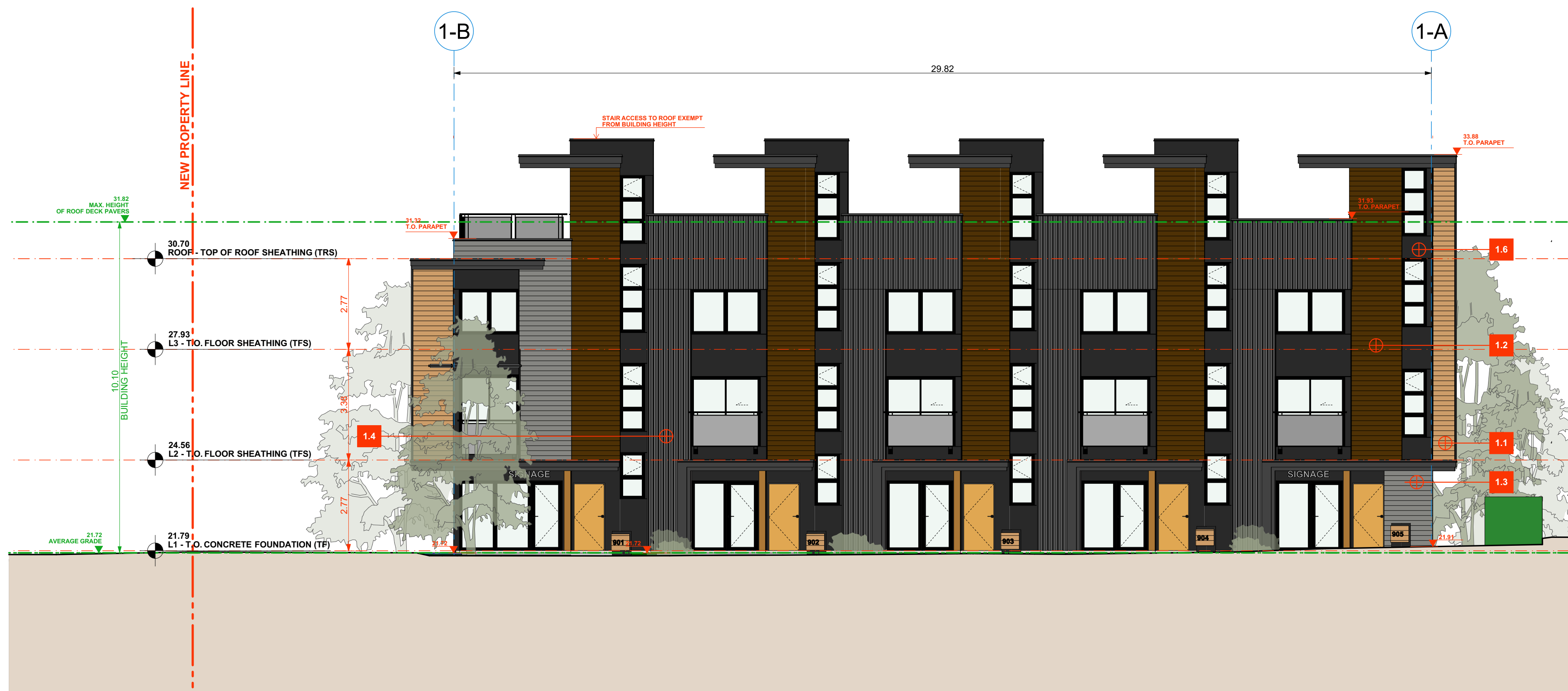
3 Building 9 - East Elevation SCALE: 1/8" = 1'-0"
