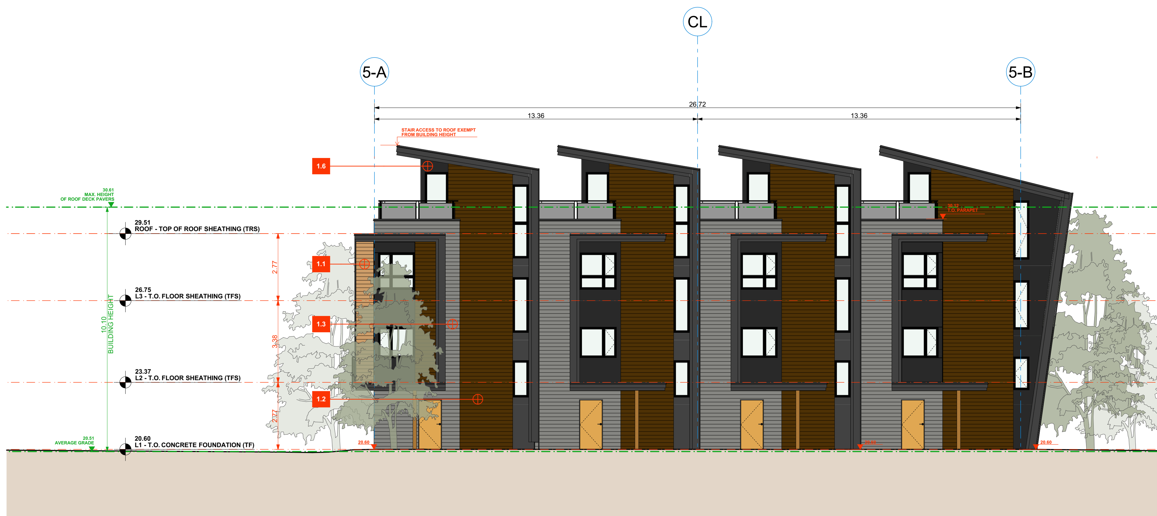
3 Building 4 - West Elevation SCALE: 1/8" = 1'-0"
