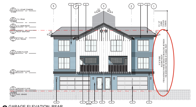
2 GARAGE ELEVATION: REAR 1/8"= 1'-0"
