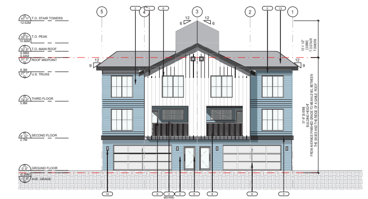
2 GARAGE ELEVATION: REAR 1/8" = 1'-0"
