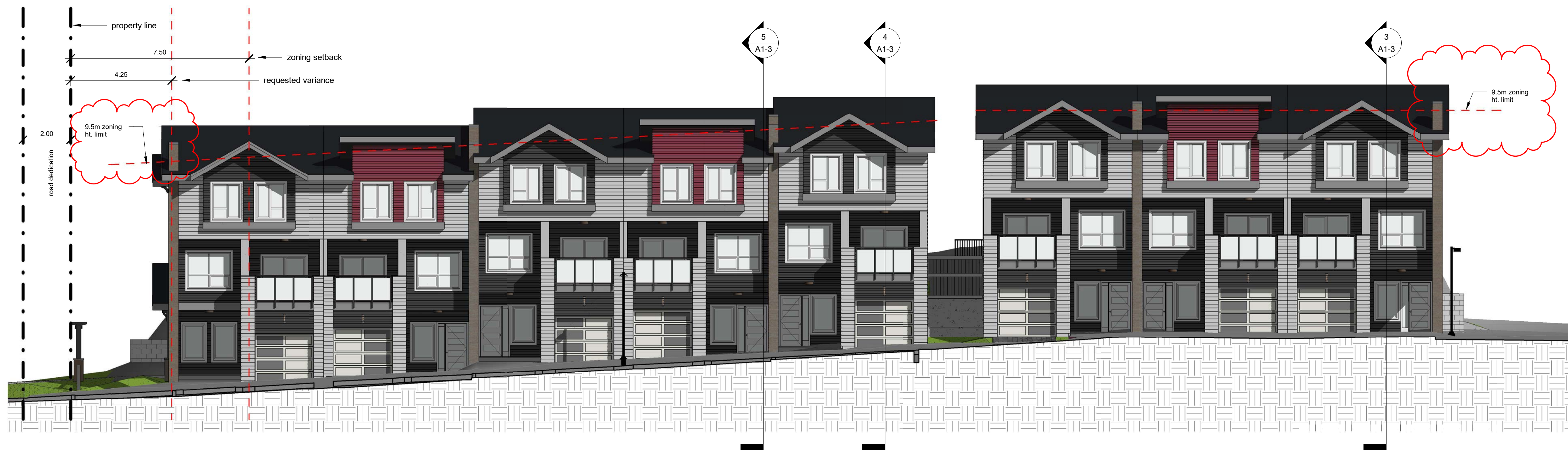
② west elevation - blocks A & B 1 : 100
